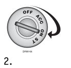
Insert the ignition key and turn it to the ON (not the START) position.
